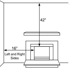
Figure 4 - Minimum Clearance to Wall and Ceiling
